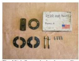
The Mitchell rear brake drum pulling tool: The two C-shaped parts (painted green on the left) are used to configure the tool to pull the shoulder and tapered design hubs. The two C-shaped parts (panted black on the right) are used to configure the tool to pull the grooved designed hubs.
